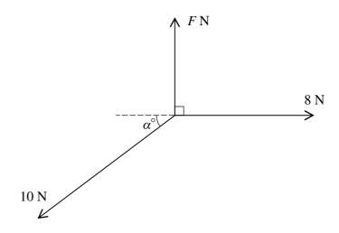
Three horizontal forces of magnitudes F N, 8 N and 10 N act at a point and are in equilibrium. The F N and 8 N forces are perpendicular to each other, and the 10 N force acts at an obtuse angle  $(90 + \alpha)^{\circ}$  to the F N force (see diagram). Calculate
